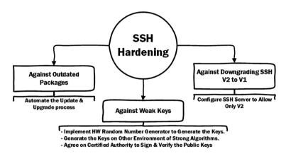
Fig. 3. Main threat sources to SSH communication and their proposed solutions.
