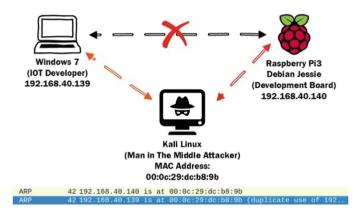
Fig. 2. Kali Linux machine acted as a MiTM to sniff the packets in both directions.
